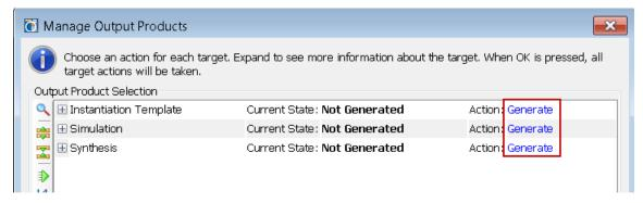
If the Generate drop down menu option is selected for the Instantiation Template, after OK is clicked, the menu will generate the .veo and related files. Pay attention to the Output product location at the bottom of the menu. These files are accessible through the IP Sources tab. Here is an example of the .veo file content.
