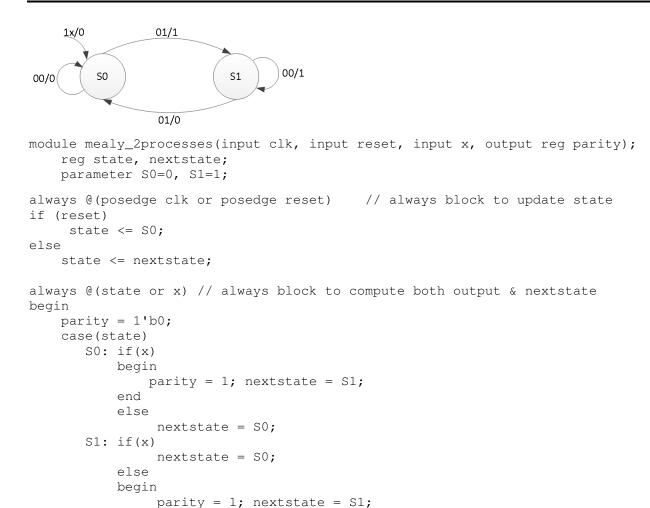
The three blocks Mealy machine and the associated model are shown below.
