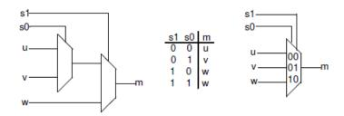
In the above diagram, u, v, w are data inputs whereas S0, S1 are select signals, and the output is m. It uses two instances of 2-to-1 multiplexer.
