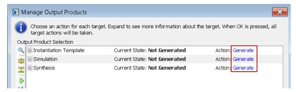
If the Generate drop down menu option is selected for the Instantiation Template, after OK is clicked, the menu will generate the .VHO and related files. Pay attention to the Output product location at the bottom of the menu. These files are accessible through the IP Sources tab. The .VHO file is the VHDL instantiation template for the generated IP. Here is an example of the .VHO file content:
