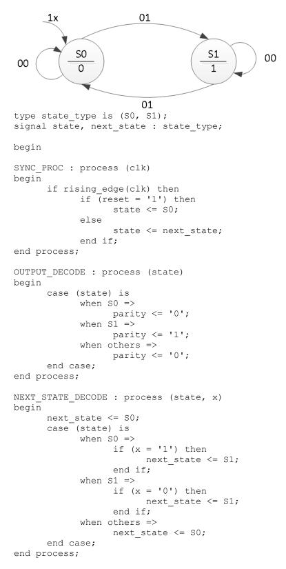
2-1. Design a sequence detector implementing a Moore state machine using three always blocks. The Moore state machine has two inputs (ain[1:0]) and one output (yout). The output yout begins as 0 and remains a constant value unless one of the following input sequences occurs:
