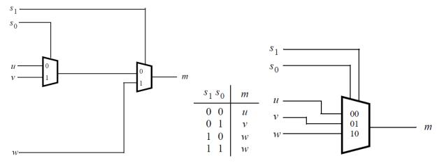
In the above diagram, u, v, w are data inputs whereas S0, S1 are select signals, and the output is m. It uses two instances of 2-to-1 multiplexer. The truth table and the top-level symbol are as provided.
