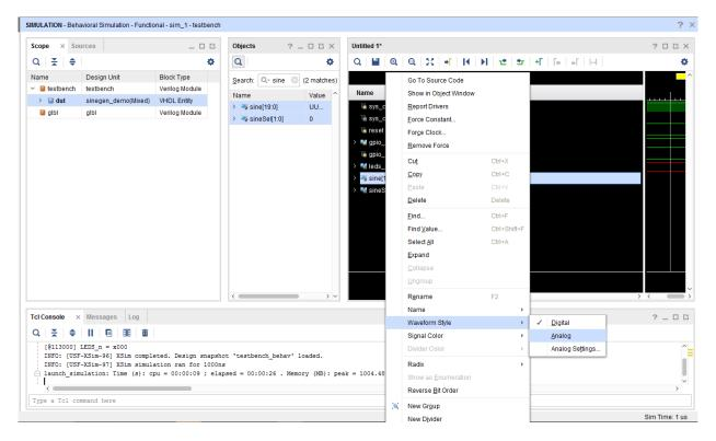
Figure 17: Enable Analog Waveform Style
