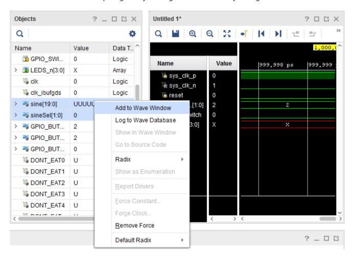
Figure 16: Add signals to Wave Window
